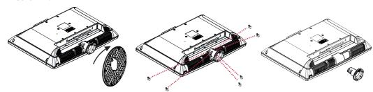
4 Attach the wall-mount bracket to your TV using the mounting holes on the back of your TV. See the instructions that came with the wall-mount bracket for information about how to correctly hang your TV.
